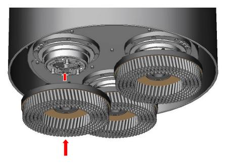
The quick clamping system can be triggered via the foot switch on the bottom of the machine casing. A simple and quick way of conducting the tool change ambidextrously.
